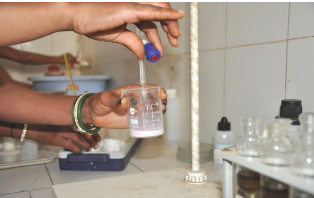
Titration test of milk underway
