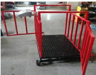
Photo b1: Detachable, Foldable and Portable Animal Loading and Unloading Ramp
